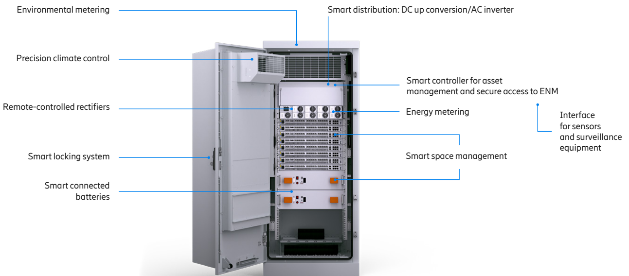
Figure 10: An overview of Ericsson Smart Connected Site
