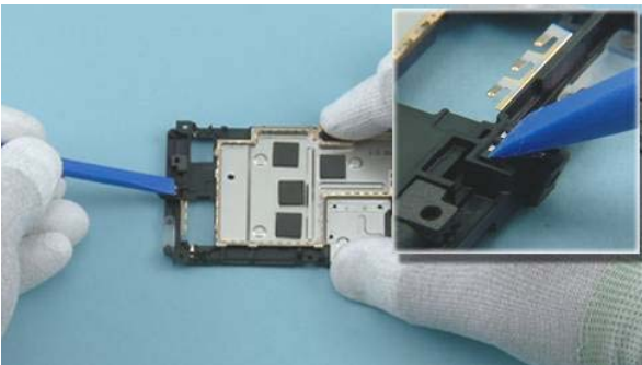
27) Insert the DC JACK with the tweezers and firmly press down on it with the SS-93 until it moves into its socket.
