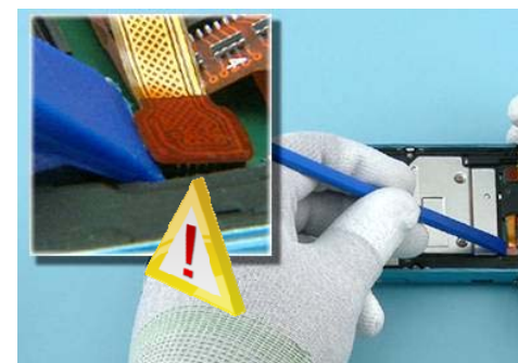
18) Use the SS-93 to open the WINDOW ASSY CONNECTOR. Be careful not to damage the connector or components nearby!
