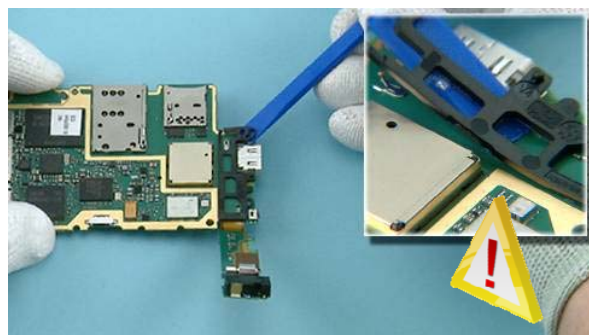
41) Use the SS-93 to release the SUB PWB SUPPORT. Be careful not to damage the components nearby!
