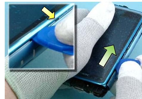
16) Release also the second clip on the other side of the phone by sliding the SRT-6 to the direction shown.
