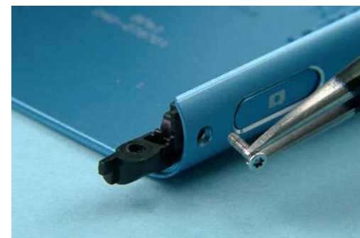
54) Remove the screw with the tweezers.
