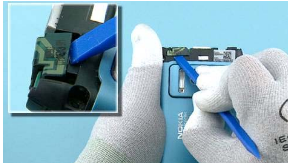
25) Release the COMBO ANTENNA with the SS-93.
